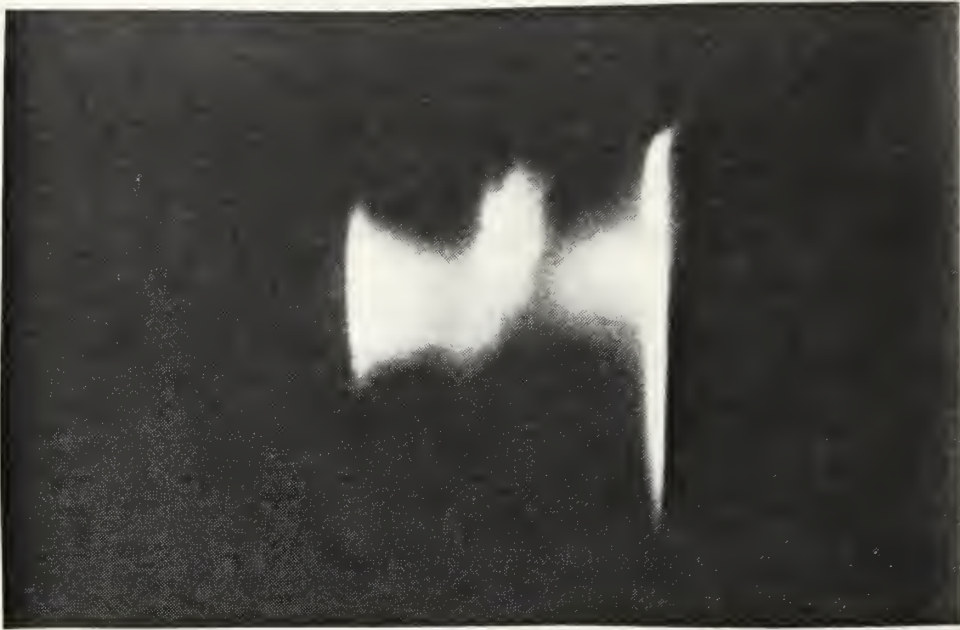
Figure 5.4 Time lapsed photograph of a 75 kV shot using a 1% neutral density filter. Notice interaction of anode and cathode plasmas.
